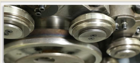
Eight-roller can sealing head can make quick replacement between 5-layer and 7-layer seal.
