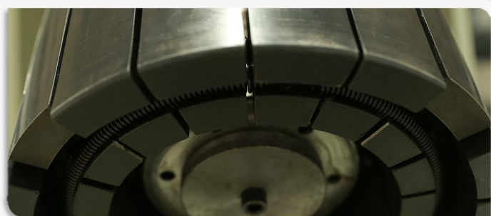
This station is all made of the high hardness, the wear-resistant import material with the function of tapering
