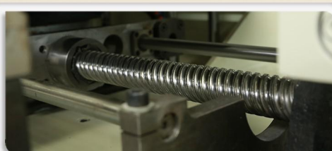
High-precision imported screw rod and servo motor are adopted to ensure the stability and rapidity of transmission
